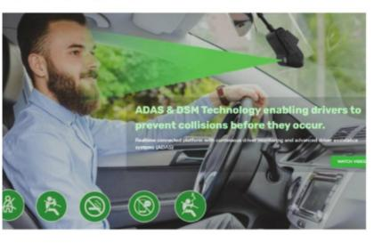
Fleetly co-pilot technology ADAS monitors road ahead and DSM camera driver's inattentiveness continuously to provide safety to vehicles and drivers. Forward facing camera monitors road conditions to avert accidents and promote safe driving by delivering in cab alerts. DSM technology monitors driver inattentiveness and provides in cab alerts to promote attentive driving.
